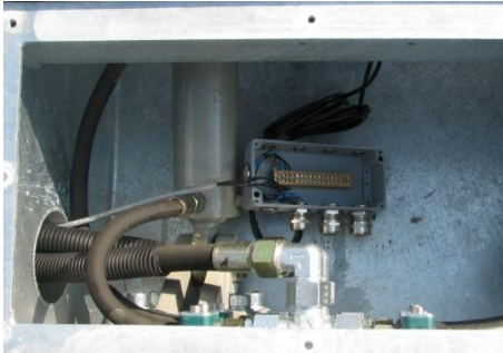
Image 9 – hydraulic line inside cylinder housing, outgoing to cabinet
