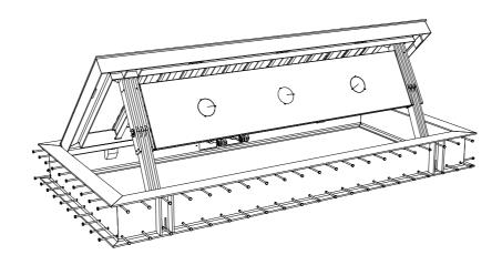
**Design:** Wedge Barrier with electro-hydraulic drive in separate drive cabinet
