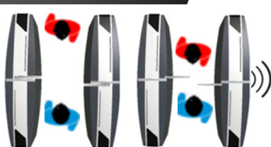
Wrong way direction/intrusion attempt
