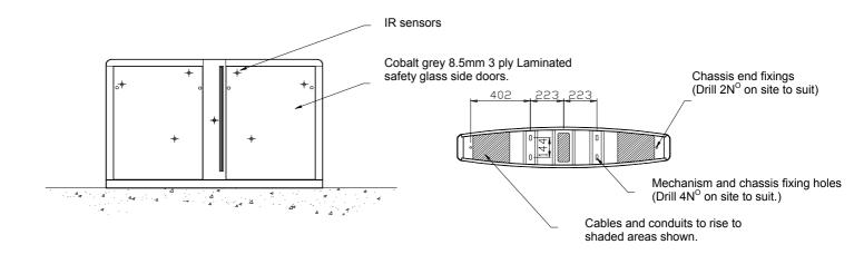
Concrete to BS 5328:1997 specification, type ST5. Base to be flat and level to +/- 5mm over the SpeedStile footprint area. 1500 x 500 x 150 deep min, per cabinet
