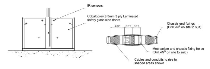
Concrete to BS 5328:1997 specification, type ST5. Base to be flat and level to +/- 5mm over the SpeedStile footprint area. 2000 x 500 x 150 deep min, per cabinet
